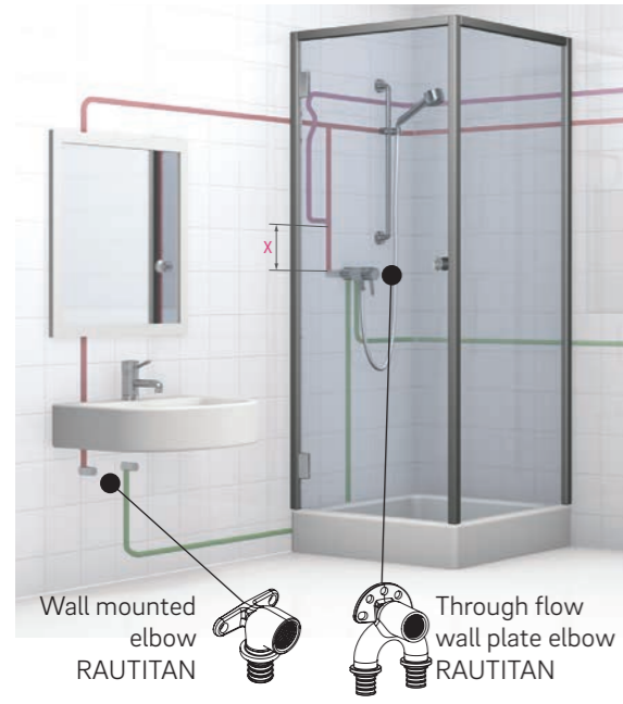
Fig. 05-4 Connection of mixer taps to pipe continuously provided with warm water - Example: Connection from top
