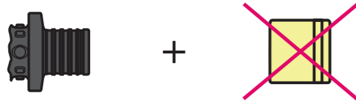
Fig. 36-1 Unapproved combination RAUTITAN PX fitting with brass compression sleeves
