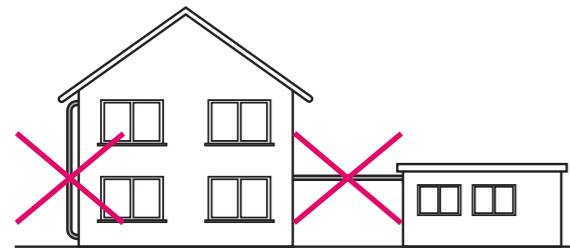
Fig. 35-7 External installations Only for water conveying pipes with adequate protective measures have been taken
