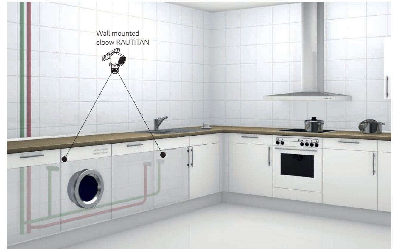
Fig. 05-2 T-piece installation with branch pipe water content < 3 l: Example kitchen
